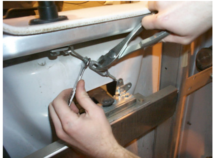
Fig. # 7 Then with a 3/8" open end wrench and a pliers you will need to adjust the turnbuckle to tighten (decrease the distance between the latch assembly and the handle).
