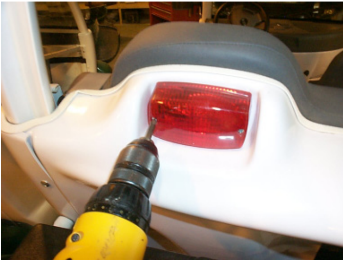
Fig. # 4 Remove (Qty. 2) screws per rear tail light cover
