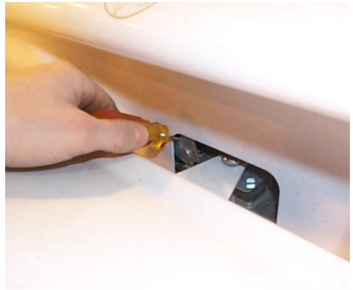
Fig. # 2 First with the latch handle in the unlocked position, try using a small flat screwdriver as shown to free the latch mechanism. Also spray WD-40 lubricant to free the parts.
