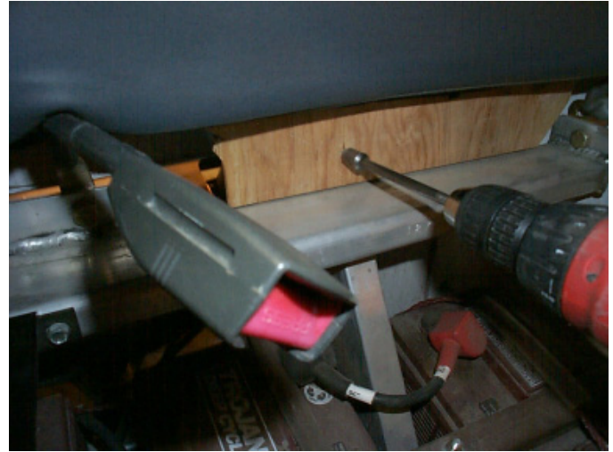
Fig. # 6 Then with a 3/8" socket, remove the 2 screws securing the seat back to the frame. Remove seat back.
