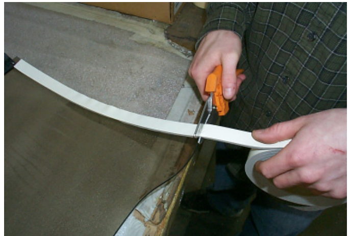
Fig. # 3 Cut vinyl foam to length.
