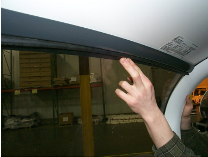
Fig. # 13 Push seal outward to form a tight seal
