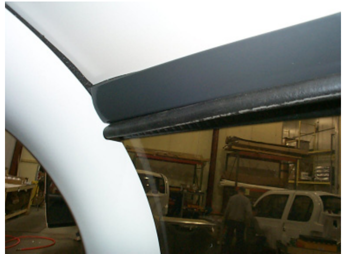
Fig. # 8 Window seal properly installed
