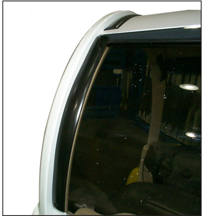
Fig. # 11 Side molding installed correctly
