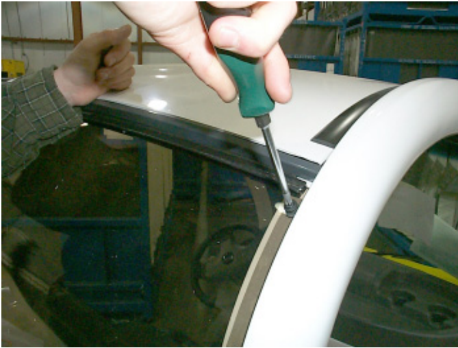
Fig. # 9 Attaching window to roof rails
