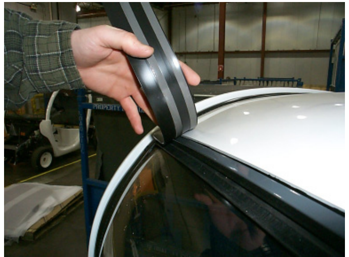
Fig. # 12 Install top molding
