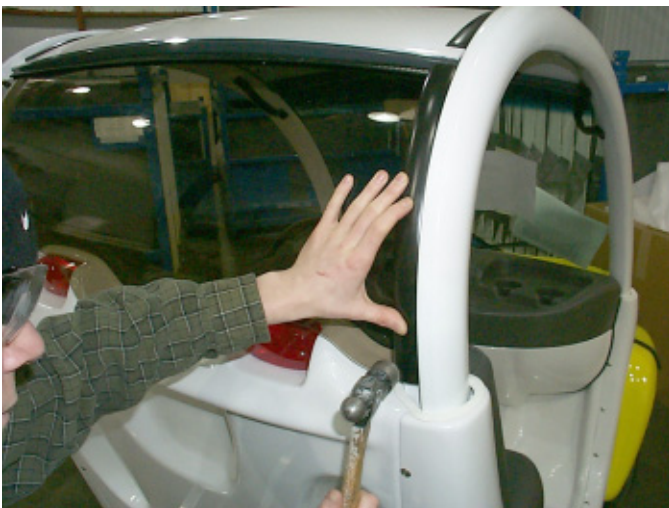
Fig. # 10 Tap molding with hammer
