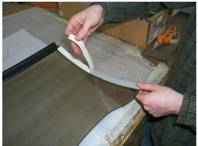
Fig. # 4 Remove backing from vinyl foam
