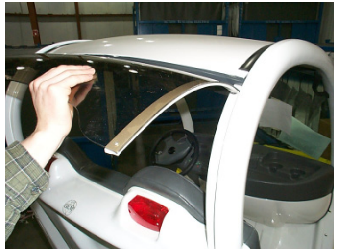
Fig. # 7 Install window seal edge first
