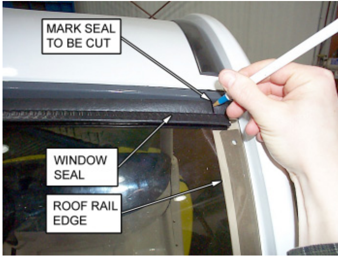
Fig. # 5 Mark the seal where it is to be cut
