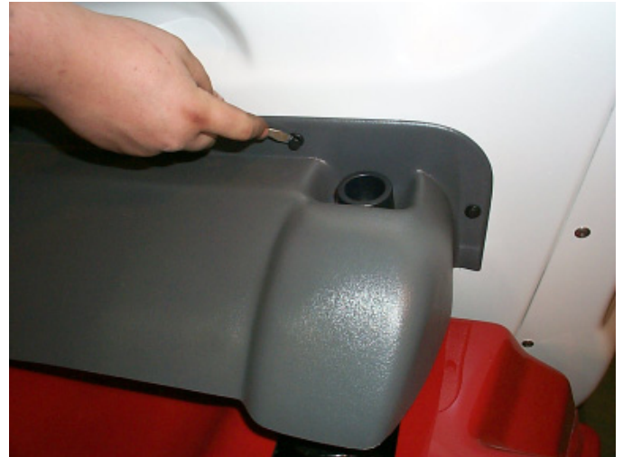
Fig. # 5 Remove rivets securing shock cover
