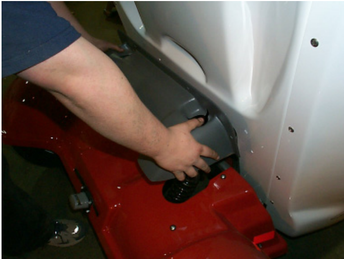
Fig. # 7 Remove shock cover
