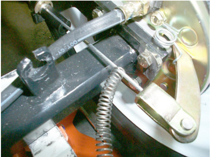
Fig. # 21 Install spring to cable
