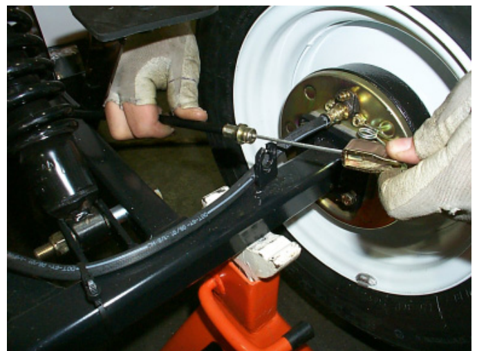
Fig. # 16 Remove parking brake cable from position
