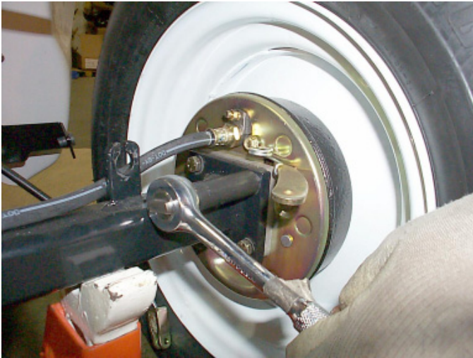
Fig. # 17 Remove rivets securing shock cover
