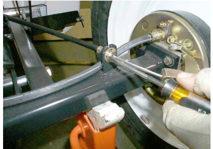
Fig. # 14 Remove e-clip securing brake line to bracket
