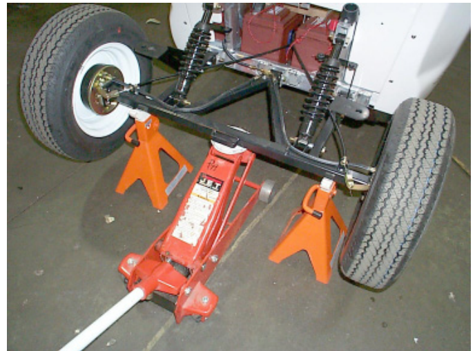
Fig. # 2 Raise vehicle to inspect
