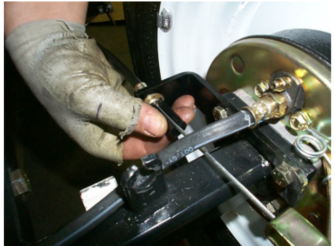
Fig. # 20 Install spacer to brake cable
