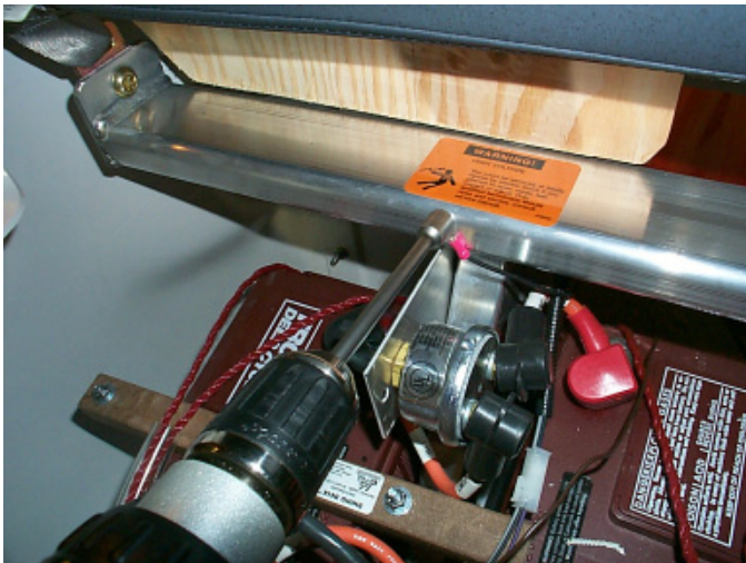
Fig. # 8 Remove ground screw
