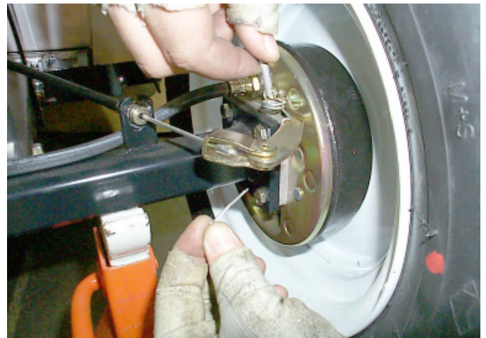
Fig. # 15 Remove cotter pin and clevis pin
