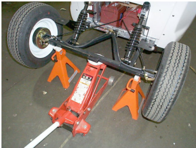
Fig. # 13 Raise vehicle to inspect
