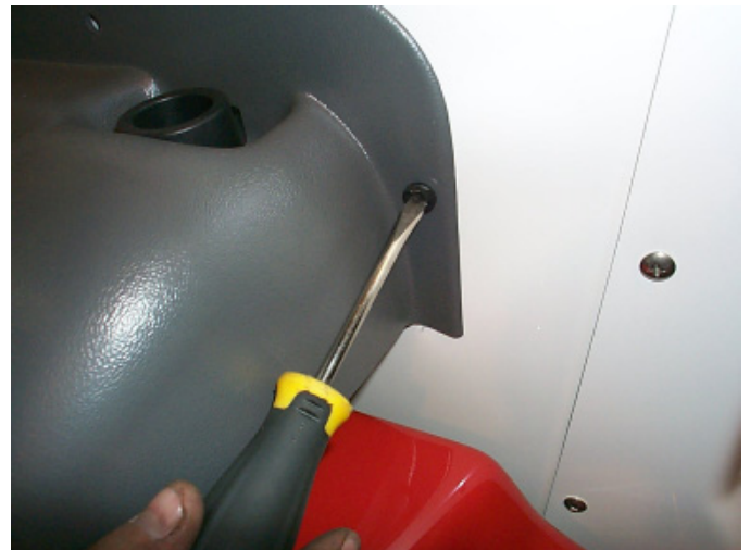
Fig. # 6 Remove rivets securing shock cover
