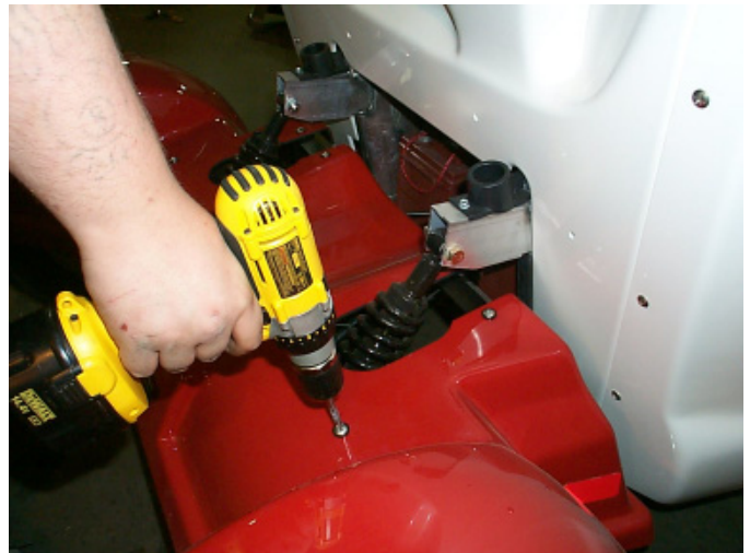
Fig. # 10 Remove screws securing spat
