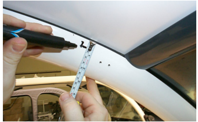
Fig. # 9 Mark and drill Ø3/8" hole in roof rail 1/2" down from ceiling
