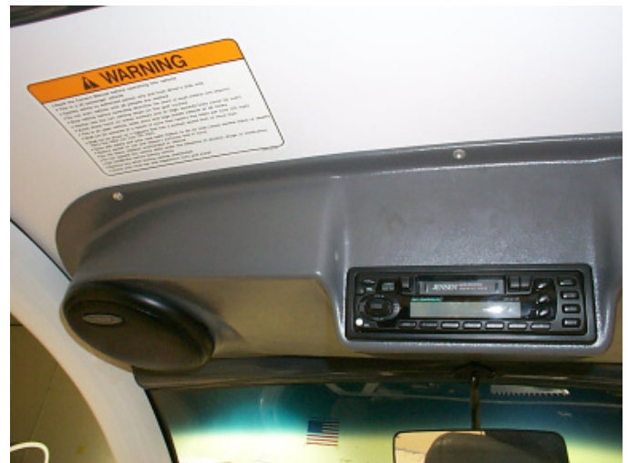
Fig. # 19 Stereo installation finished
