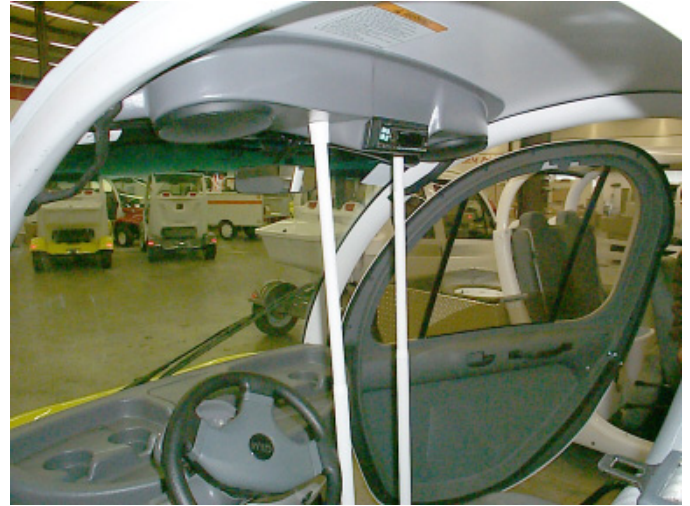
Fig. # 14 Drill lower hole in roof rail
