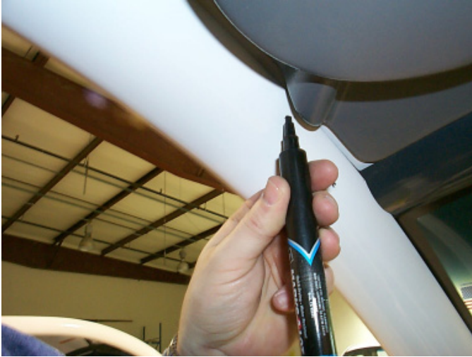
Fig. # 7 Mark hole locations for wiring harness
