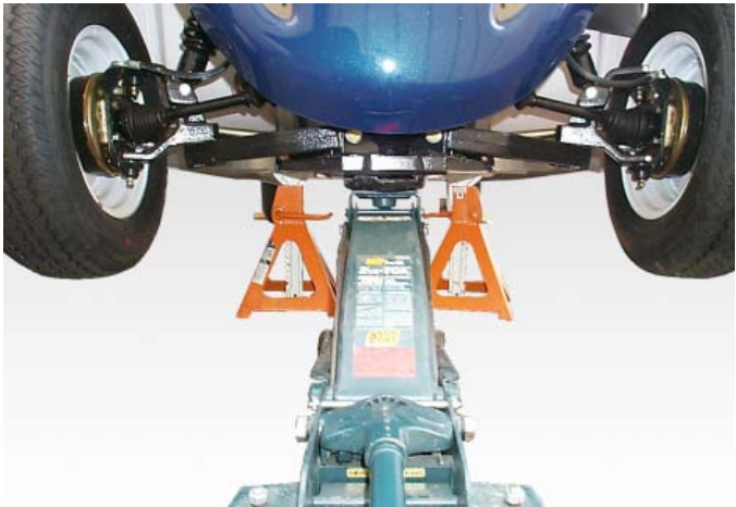
Fig. # 2 Raise vehicle with hydraulic jack.
