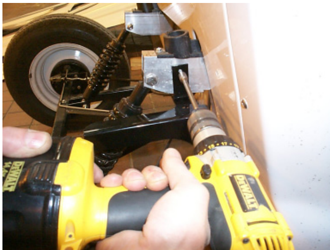
Fig. # 17 Secure spat bracket
