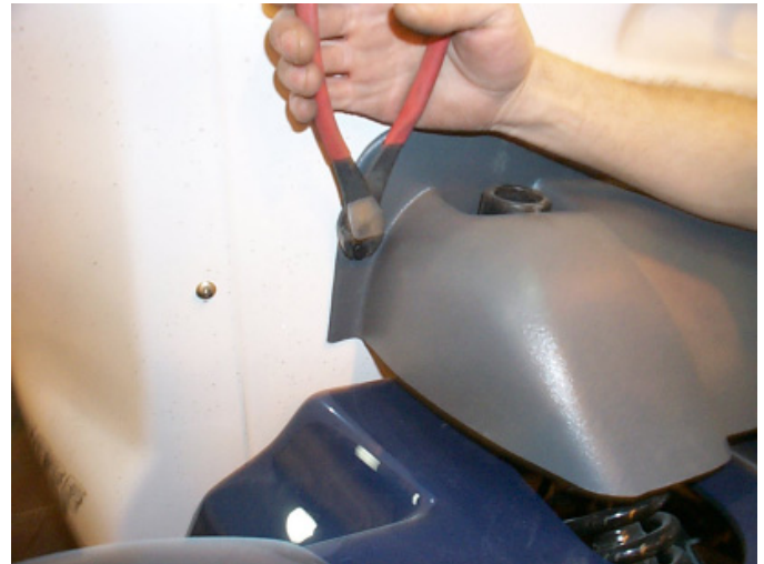
Fig. # 4 Remove the (qty. 4) push tuflok rivets securing the shock mount cover
