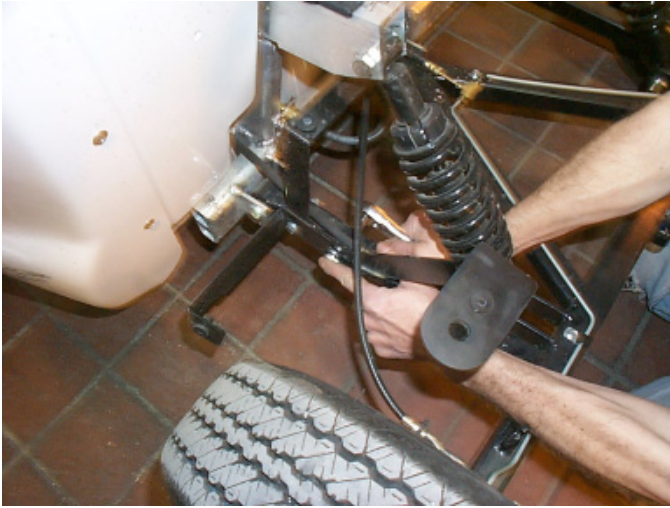
Fig. # 7 Remove and discard old spat mounting brackets
