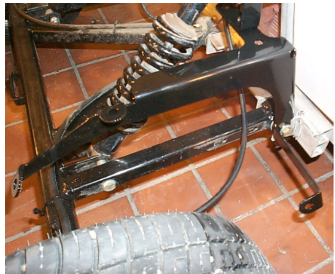
Fig. # 15 Install new spat mounting brackets
