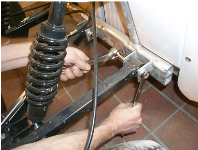
Fig. # 10 Remove bolt and nut securing rear sus. assembly to frame
